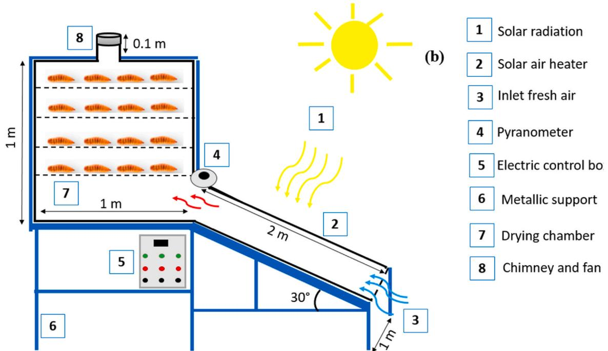
Fig. 3. (a) Real picture of the dryer, (b) 2D schematic of the hybrid solar-electrical dryer.
