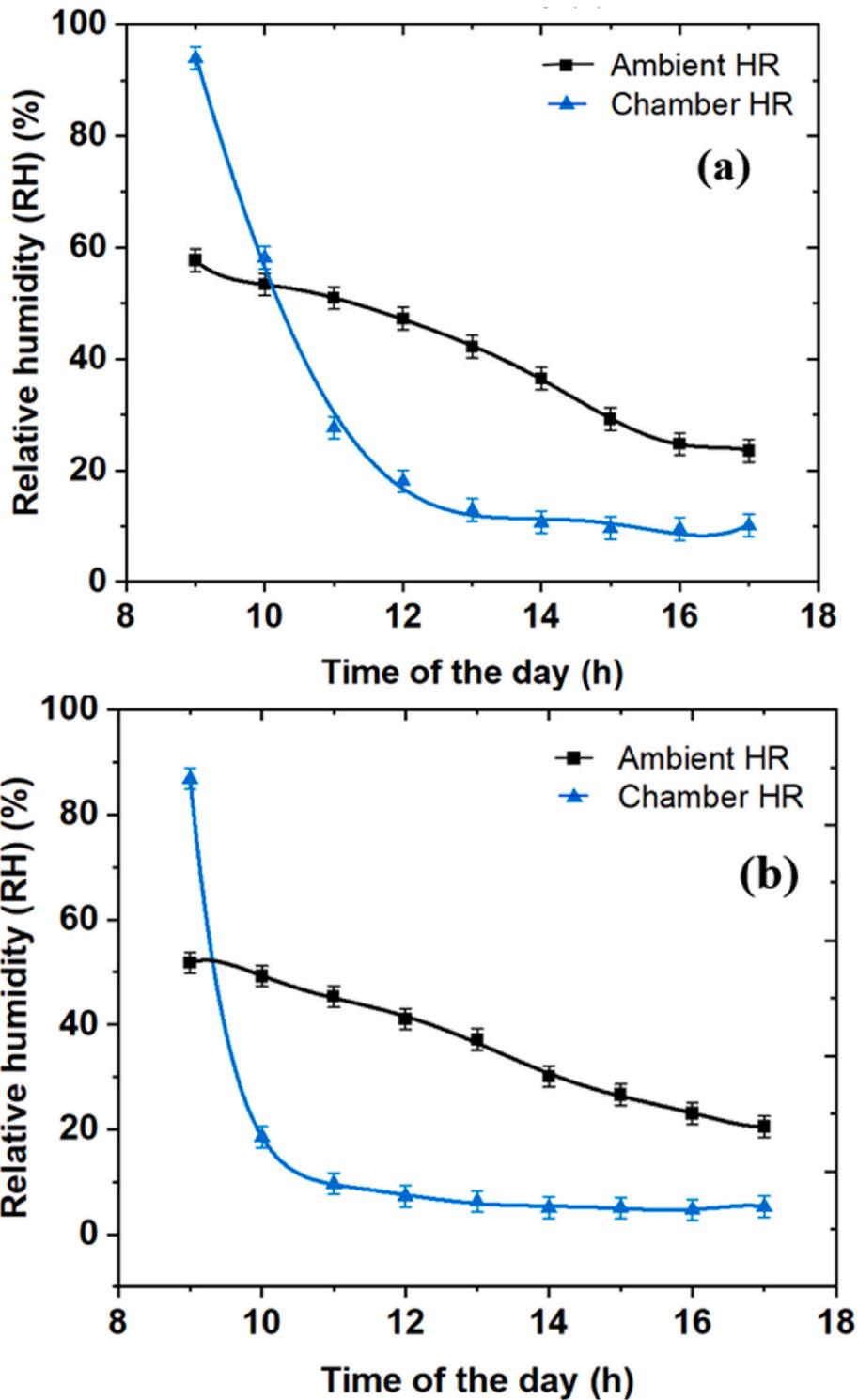
Fig. 7. Variation of ambient and drying chamber relative humidity over time: (a) solar mode, (b) hybrid mode.
