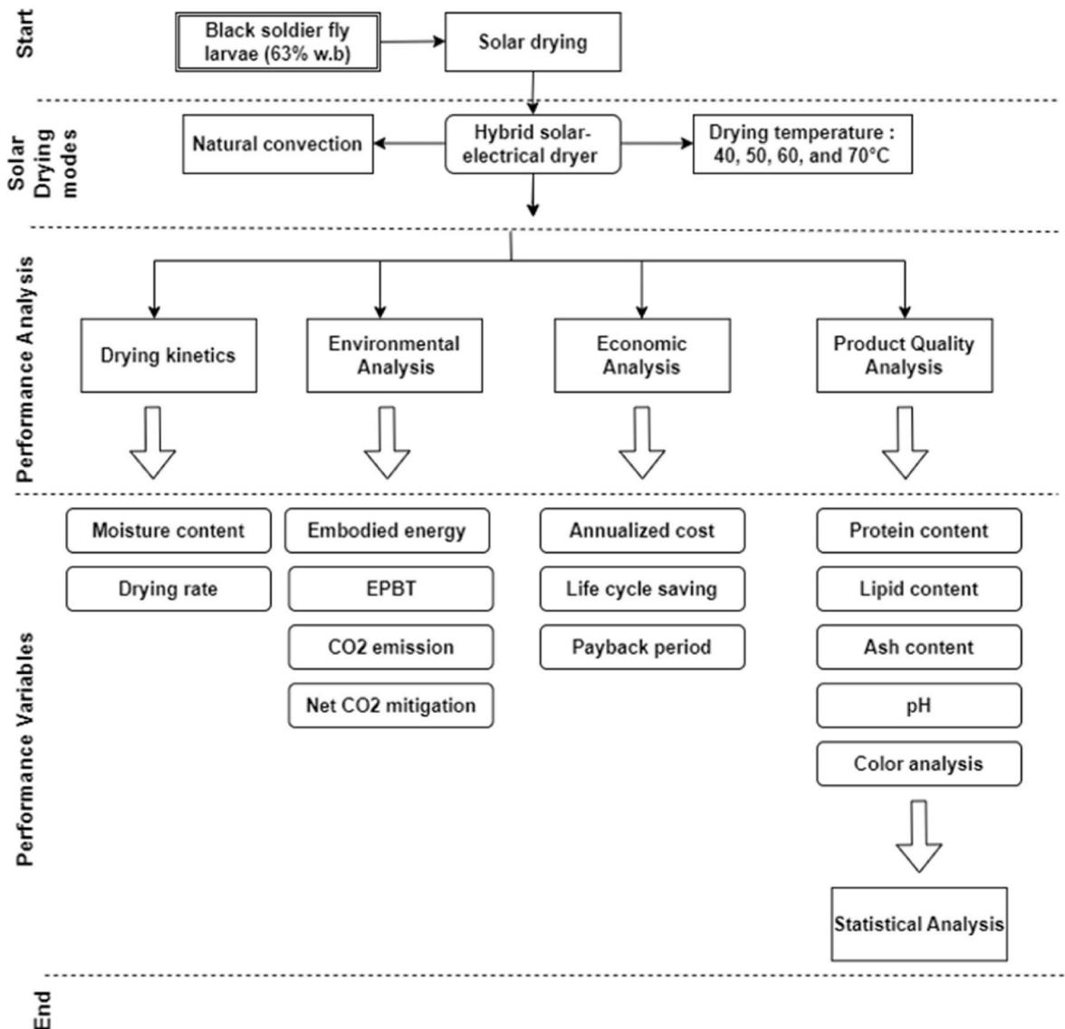
Fig. 4. Block diagram representation of the experimental methodology.
