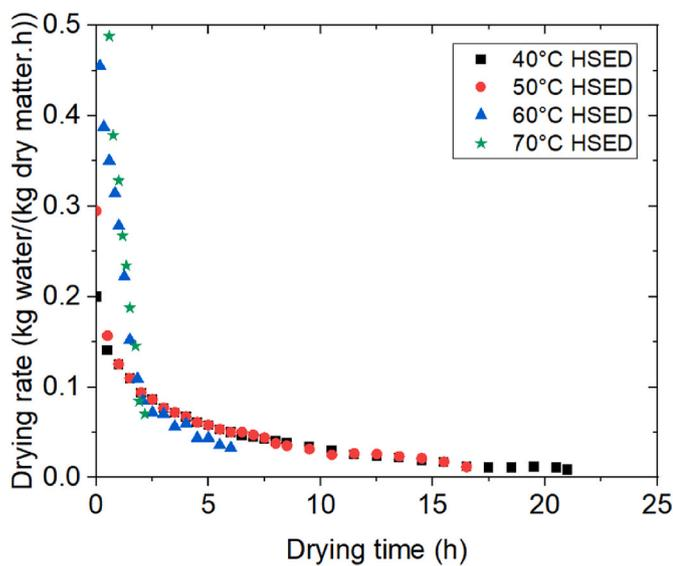
Fig. 9. Evolution of drying rate of black soldier fly larvae over drying time.
