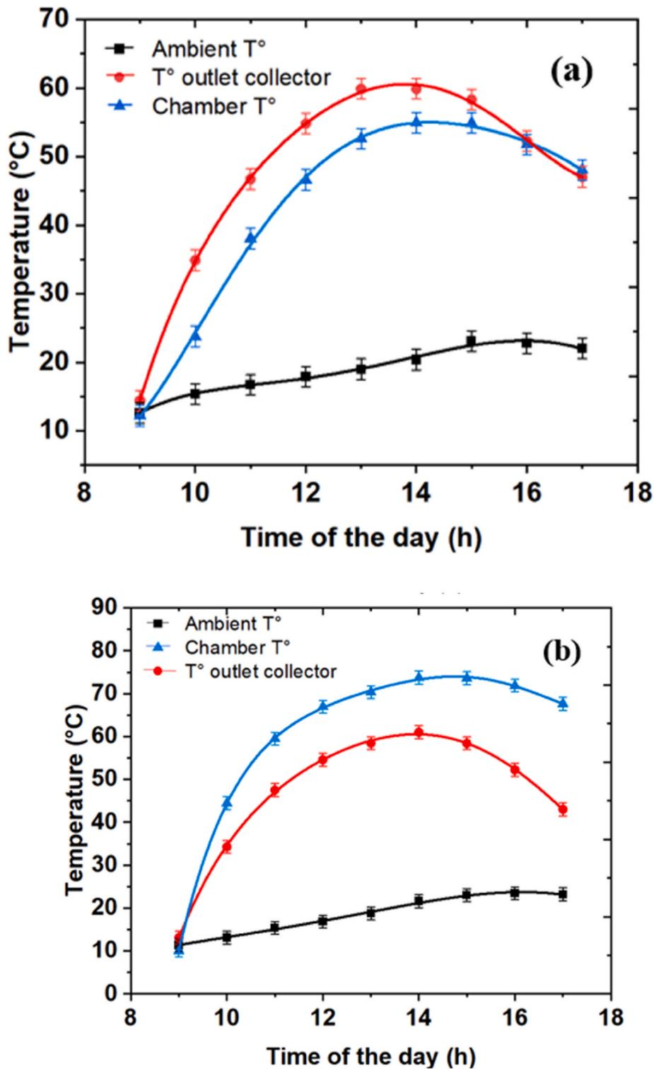
Fig. 6. Variation of ambient temperature, drying chamber temperature, and the temperature at the outlet of the collector over time: (a) solar mode, (b) hybrid mode.
