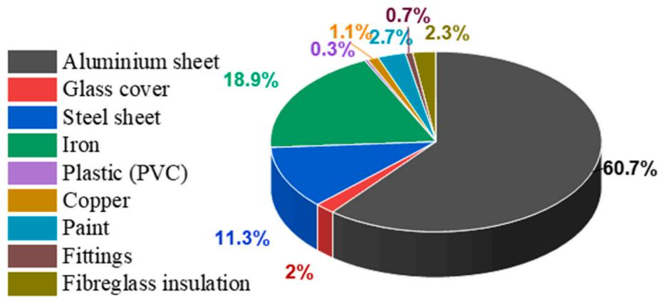
Fig. 11. Pie chart of the embodied energy of materials used for the design of the hybrid solar-electrical dryer.
