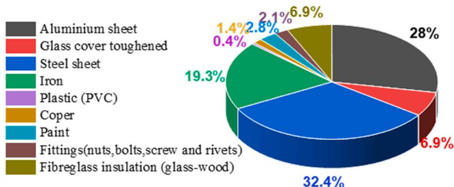
Fig. 10. Pie chart of the masses of materials used for the design of the hybrid solar-electrical dryer.
